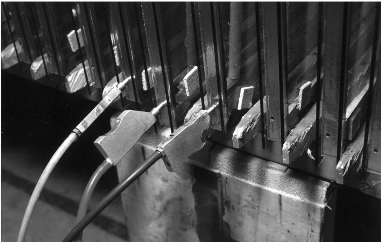
Argon gas being added to sealed window units.
